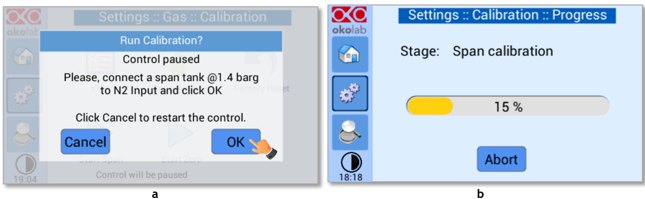
Figure 43. Span calibration running (a – b)
