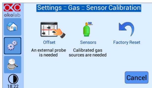
Figure 31. How to enter a gas offset calibration.
