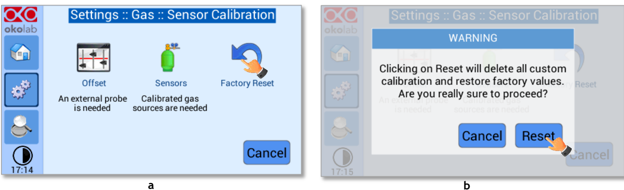
Figure 46. Sensor calibration factory reset (a - b).
