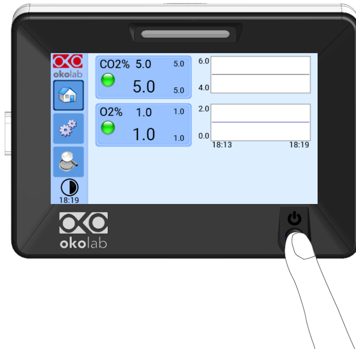
Figure 81. How to enter in Touch Screen Calibration.
